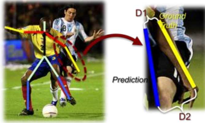
Figure 3.4: Illustration of distances D1 and D2 , the two measurements involved in evaluating body part localizations (see text). The first measure of PCP considers a part correctly localized if both distances are below a threshold, whereas the second measure considers a part correctly localized if the mean of D1 and D2 is below a threshold.
