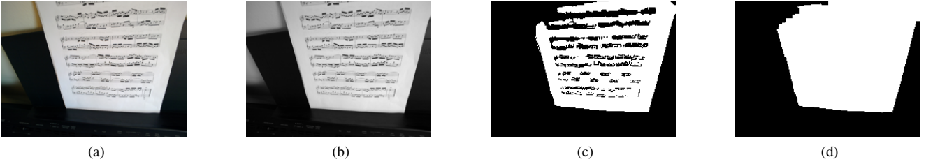
Figure 2: Proposing candidate score region: (a) color image down-sampled to 1/10 its original size; (b) converted to grayscale; (c) thresholding and binarization; (d) morphological smoothing and hole-filling.
